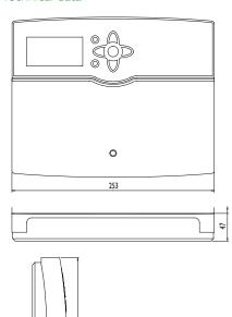
**Inputs:** 12 Pt1000, Pt500 or KTY temperature sensor inputs (can optionally be used for remote controls, operating mode switches or potential-free switches), 3 impulse inputs for V40 flowmeters, 1 input for a FlowRotor, 1 CS10 solar cell, 4 Grundfos Direct Sensors  $^{\text{TM}}$  (2 x analogue, 2 x digital\*)
